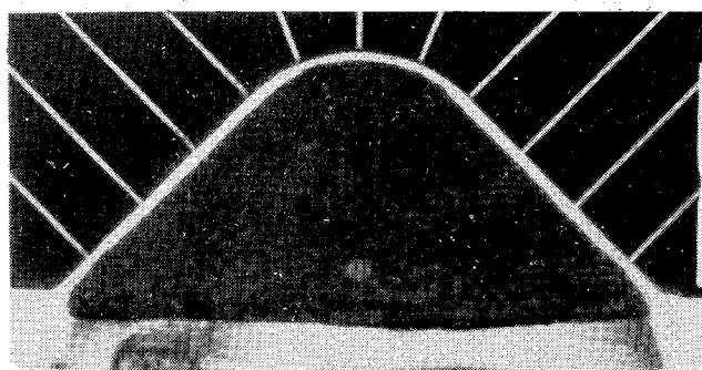
Fig. 3 Post-test model contour in relation to pretest contour represented by a template, shot 5471.
